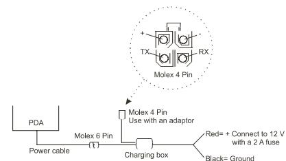
See the back of this leaflet to find the correct adapter to connect to the Molex connector.
